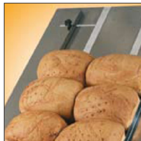
High-capacity ramp featuring side guides and shoes. Used to store and deliver loaves to the slicer.
