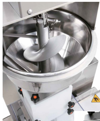
The MultiForm's dual hopper design accommodates both filling and crust.
