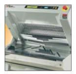
The PicomaticONE can easily slice large round loaves. Once cut the slices are held by the flaps.
