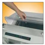
When closed, the rear safety lid triggers start-up. It opens automatically when slicing is complete.
