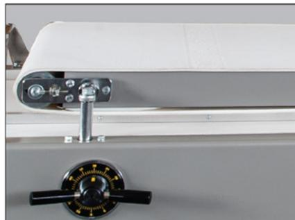
Motorized Moulding Plate with Fine Height Adjustments
